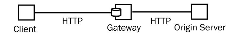
The use of a gateway (or reverse proxy) is imposed by the server
