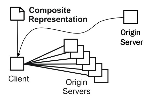
A composite representation is interpreted by the client that follows its hyperlinks and aggregates the state of the referenced component resources
