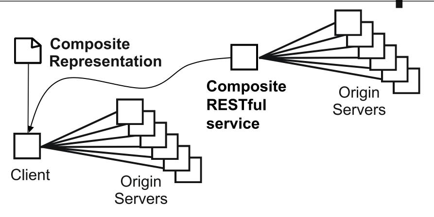
A composite representation can be produced by a composite service too
